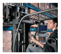
Pickers can be armed with a handheld mobile computer that has bar code scanning and a real-time wireless connection to your business systems to dramatically streamline the picking process.
