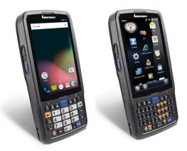
With its multi-touch, outdoor-readable screen, long battery life and highly accurate barcode scanning capabilities, the CN51 Mobile Computer offers unparalleled versatility and performance for mobile workers.
